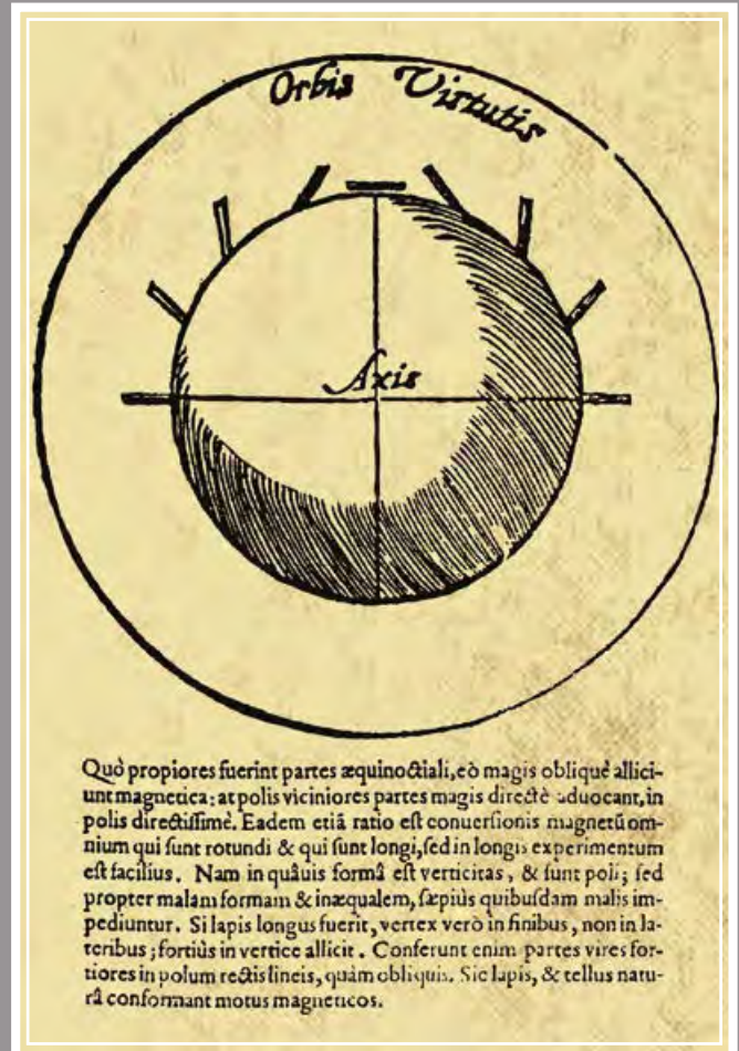
Demonstration of the behaviour of the magnetic poles through the "Terrella", a miniaturized model of the Earth and the field generated by the same, created by William Gilbert [1544-1603], the first magnetism scholar
